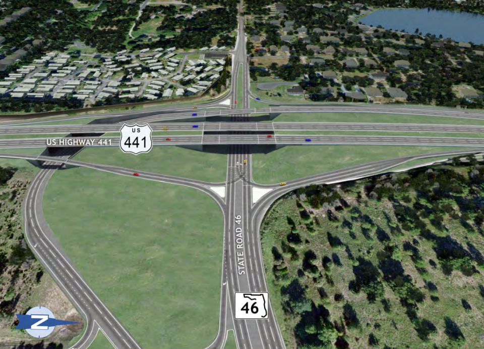
GRADE SEPARATED INTERSECTION WITH DUAL LEFT TURNS – WESTBOUND VIEW
