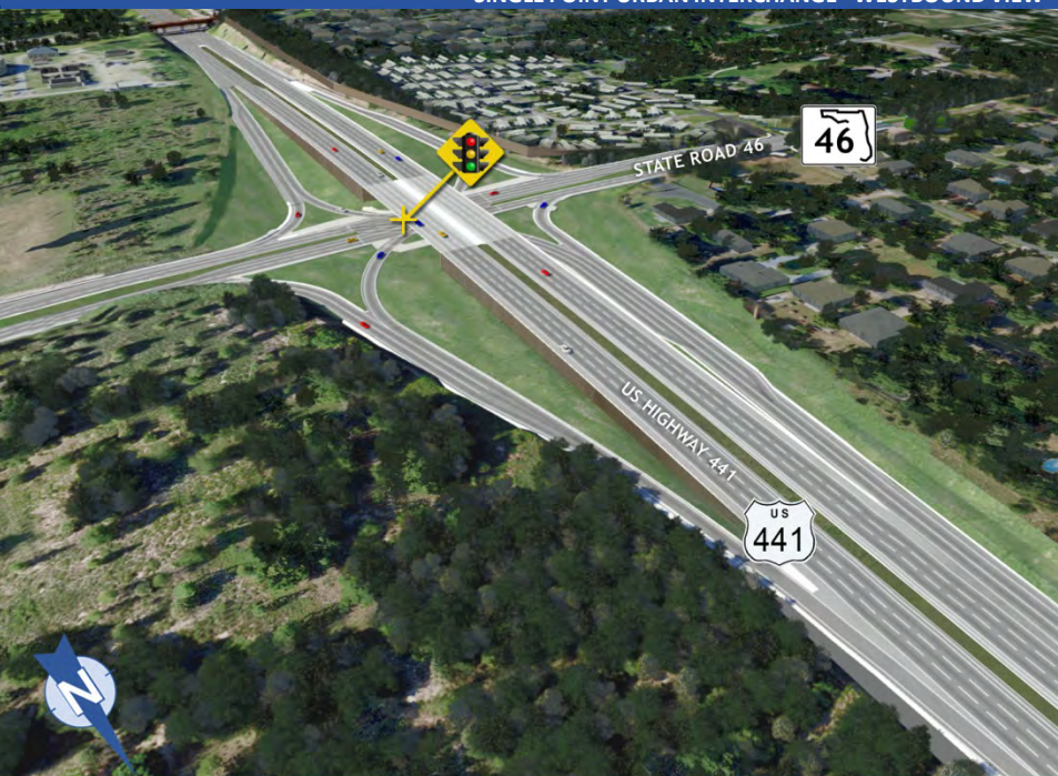
SINGLE POINT URBAN INTERCHANGE – BIRD'S EYE VIEW
