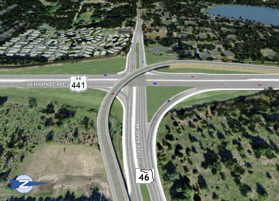
AT GRADE INTERSECTION WITH FLY-OVER BRIDGE – WESTBOUND VIEW
