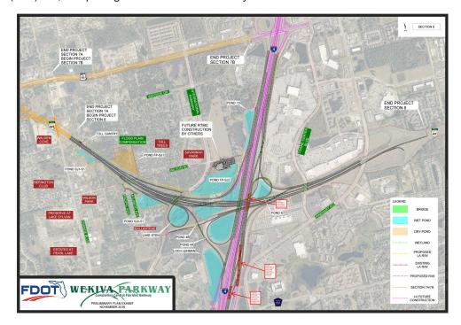
Section 8 involves building the parkway from Orange Boulevard to east of Rinehart Road in Sanford. This section includes building the general use lanes for the future I-4 Beyond the Ultimate project, from south of S.R. 417 to south of S.R. 46. The parkway will include aesthetic walls and other features. A toll gantry will be built on this section.
