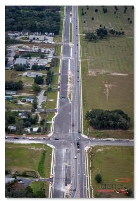
The first half of 2019 saw widening come to a completion of the S.R. 46 corridor to the north throughout the project limits. Paving operations in the spring allowed crews to shift all S.R. 46 traffic to the future westbound lanes so that similar widening could be performed on the south side of the corridor. Work on the south side included earthwork, drainage and paving.
