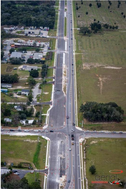
The first half of 2019 saw widening come to a completion of the S.R. 46 corridor to the north throughout the project limits. Paving operations in the spring allowed crews to shift all S.R. 46 traffic to the future westbound lanes so that similar widening could be performed on the south side of the corridor. Work on the south side included earthwork, drainage and paving.
